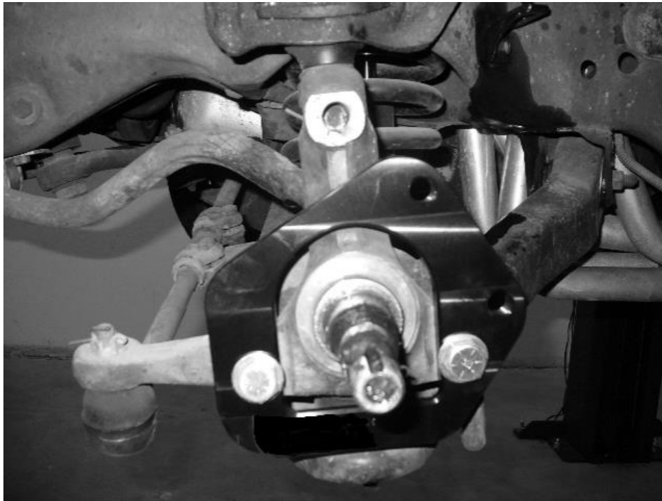
Figure 2 – Primary Caliper Mounting Bracket (Driver Side shown for A-body application)
