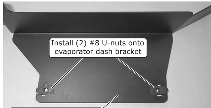
Evaporator Dash Bracket 640710
