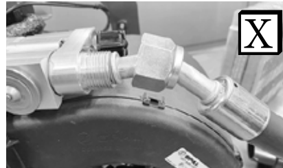
Improperly Seated O-ring Land
