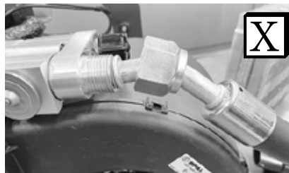
Improperly Seated O-ring Land
