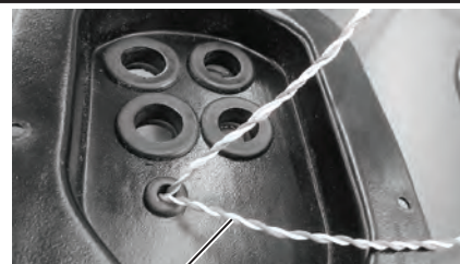
Route red, white and blue wires from main harness through 7/8" wiring grommet on kick panel cover
