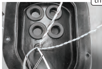
Route heavy gauge orange and white wires through 7/8" wiring grommet on kick panel cover
